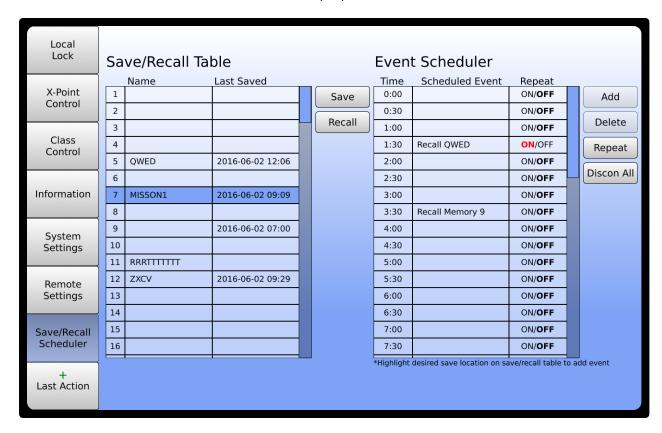
To save or recall a configuration, use the scroll bar on the right hand side to locate the desired numerical memory location. Touch the line item to highlight it, then select the save button to save the configuration or the recall button to recall a saved configuration. In either case, a confirmation window will appear prompting the user to confirm the action.
